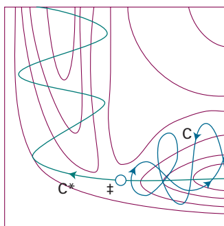
Fig. 22.24 An attractive potential energy surface. A successful encounter ( C^* ) involves high translational kinetic energy and results in a vibrationally excited product.
