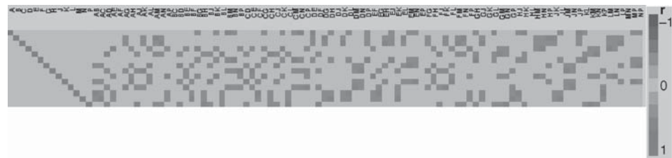
■ FIGURE 9.20 Correlations of main effects and two-factor interactions, no-confounding design for 14 factors in 16 runs
